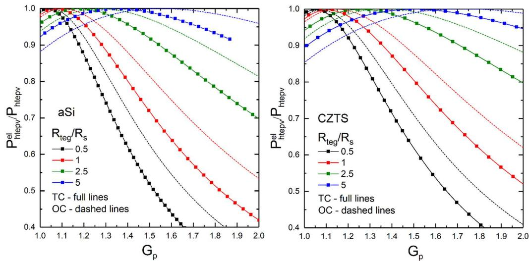
**Figure 4.** Interplay between electrical losses and  $G_p$  for a-Si (left) and CZTS (right) solar cells. In both graphs full and dashed lines represent the case of TC and OC systems respectively, while the different colors stand for different  $R_{i,teg}/R_s$  ratios. Simulations were run varying  $T_{cell}$  between 300 and 500 K with 5 K steps (squares highlight the temperature steps).
