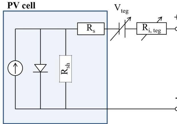
**Figure 1.** Scheme of the simulator used in this work. Several PV cells were connected in series with a voltage generator and a variable electrical resistance.
