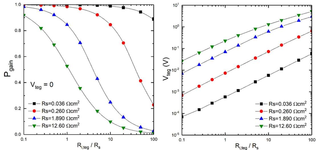
**Figure 3.** (Left) Effect of  $R_{i,\text{teg}}$  on the solar cell power in the case of  $V_{\text{teg}} = 0$ . (Right)  $V_{\text{teg}}$  needed for lossless condition.
