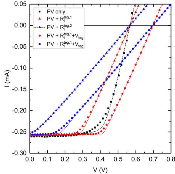
**Figure 2.** Example of the effect of  $R_{i,teg}$  (red and blue triangles) and the combination of  $R_{i,teg}$  and  $V_{teg}$  (red and blue circles) on the IV curve of a solar cell (black squares). Dashed lines are the fits calculated by Eq. 7. In this example  $R_{i,teg}^1 < R_{i,teg}^2$ .
