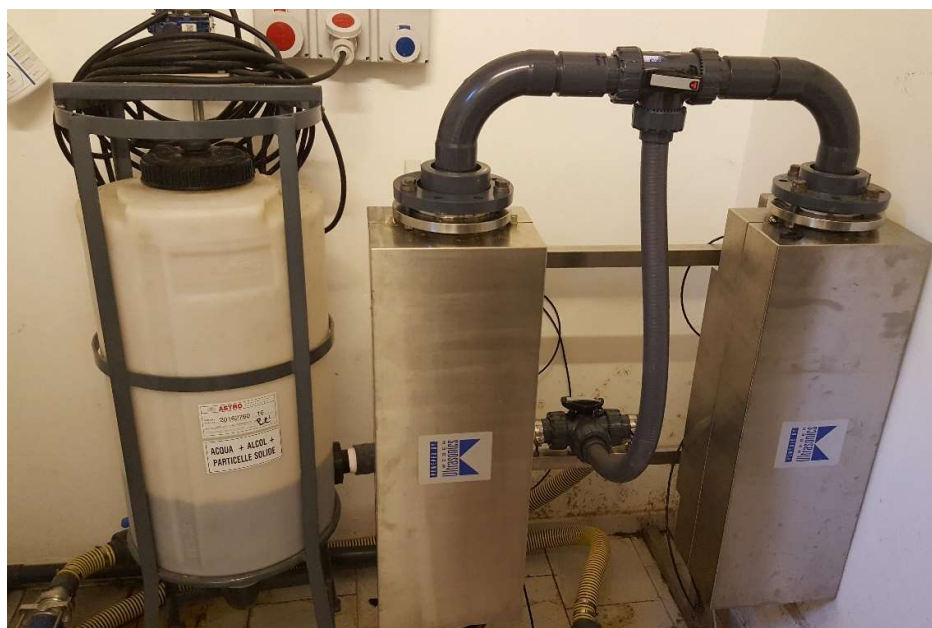
Figure 5. Double-unit, high-power sonochemical reactor (25 kHz and multi-frequency 80-120 kHz) ("green technologies development platform" DSTF -University of Turin).
