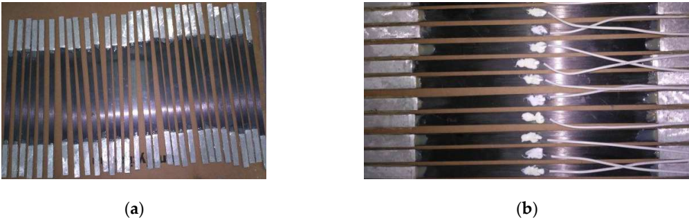
Figure 4. Photograph of the coupons: (a) CFRP plate coupon; (b) the location of strain gauge.
