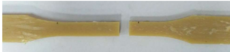
Figure 9. Failure mode of the epoxy adhesive coupon under tension.
