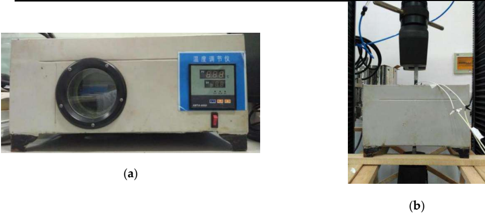
Figure 5. Test setup: (a) temperature chamber; (b) specimens setup.
