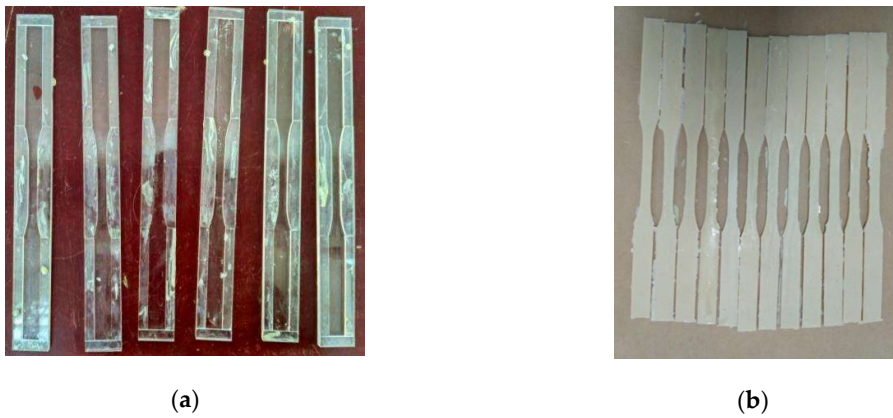
Figure 2. Photograph of the specimens: (a) plexiglass mold; (b) adhesive coupons.
