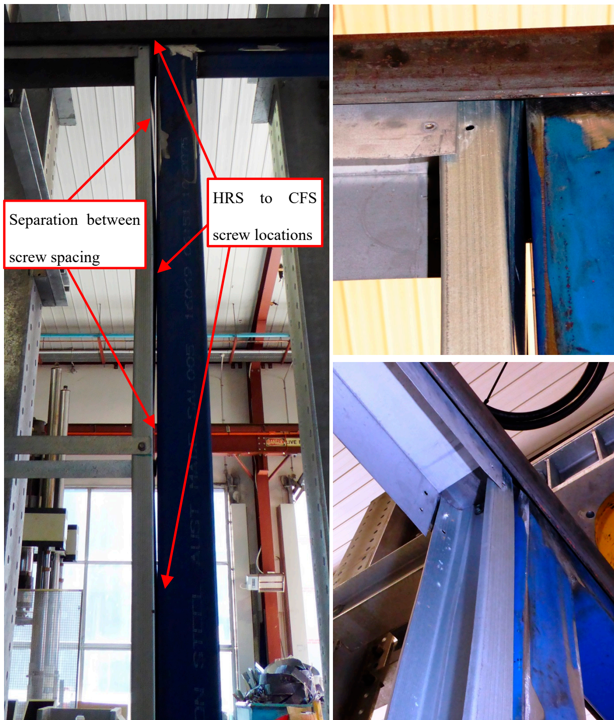
Figure 3. Local deformations and screw failure under monotonic pull load
