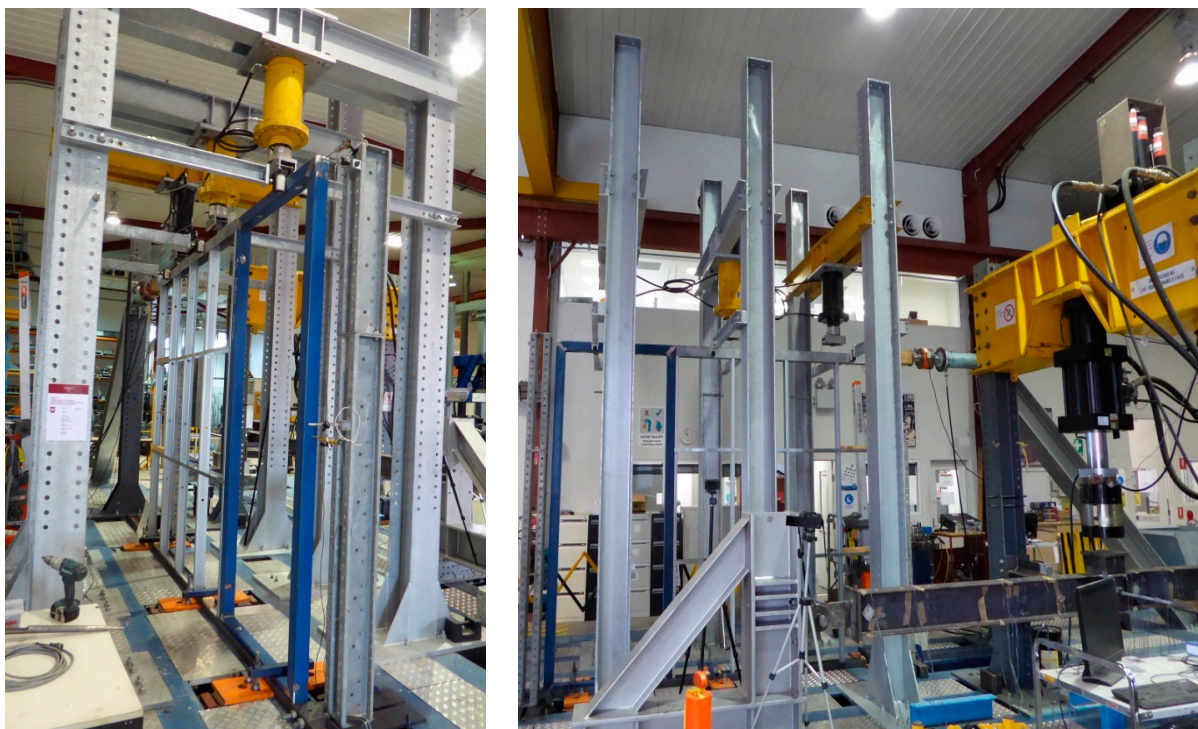
Figure 2. Fabricated test frame and specimens setup
