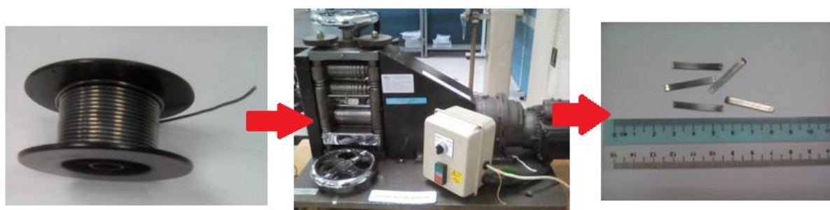
Figure 2. Filler metal preparation process
