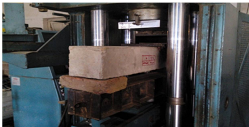
Figure 2. Three- point bending test setup in UTM
