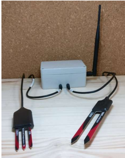
Figure 6. Node with Decagon Soil Moisture sensors.
