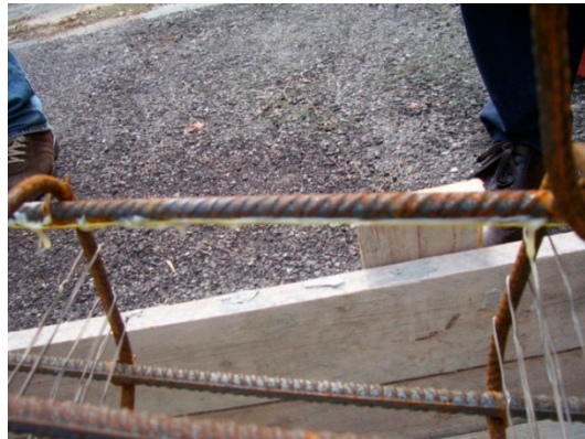
Figure 1. Fiber fixing: (a) the upper fiber is glued to the reinforcement; (b) an iron wire grid to fix the lower fibers.
