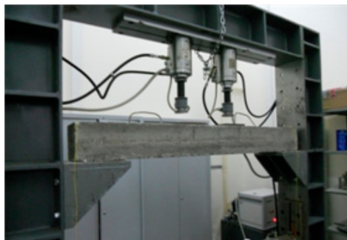
Figure 2. Testing apparatus, load frame and hydraulic jacks
