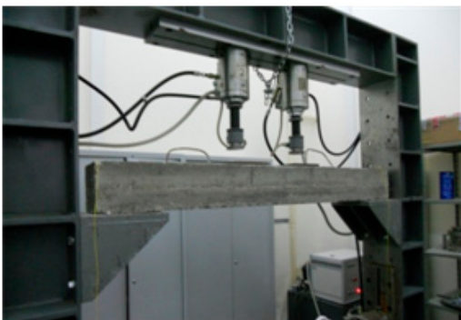
Figure 3. Testing apparatus, load frame and hydraulic jacks
