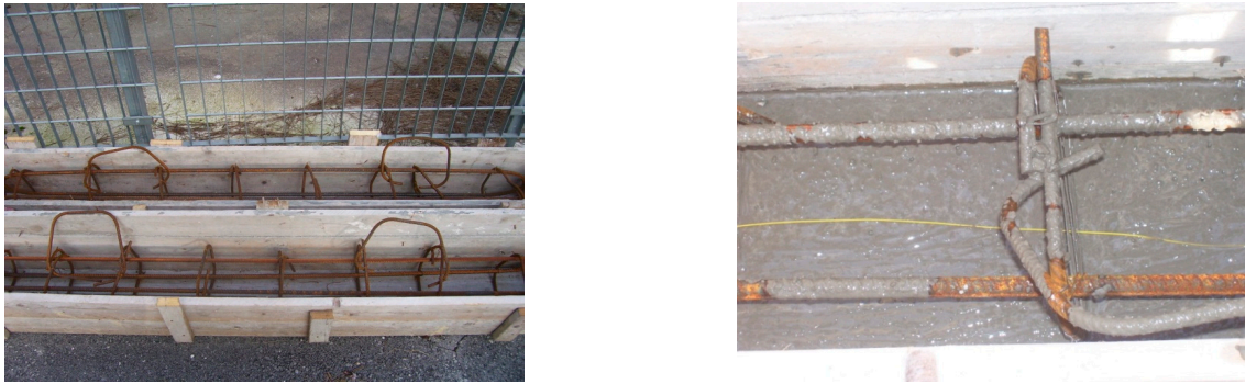
Figure 1. Building of the specimen: (a) description of the reinforcement pattern; (b) casting phase and optical fiber embedding.
