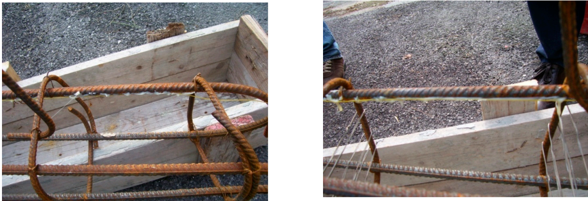
Figure 2. Fiber fixing: (a) the upper fiber is glued to the reinforcement; (b) an iron wire grid to fix the lower fibers.
