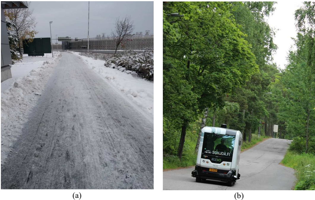
Figure 15. (a) Wintery weather stopped the operation in Helsinki pilot. The lidars of the robot bus see snow banks as obstacles. (b) An example of an area where the EZ10 robot bus localization does not work, as the trees are blocking the satellite connection and there are no fixed structures for the lidars.
