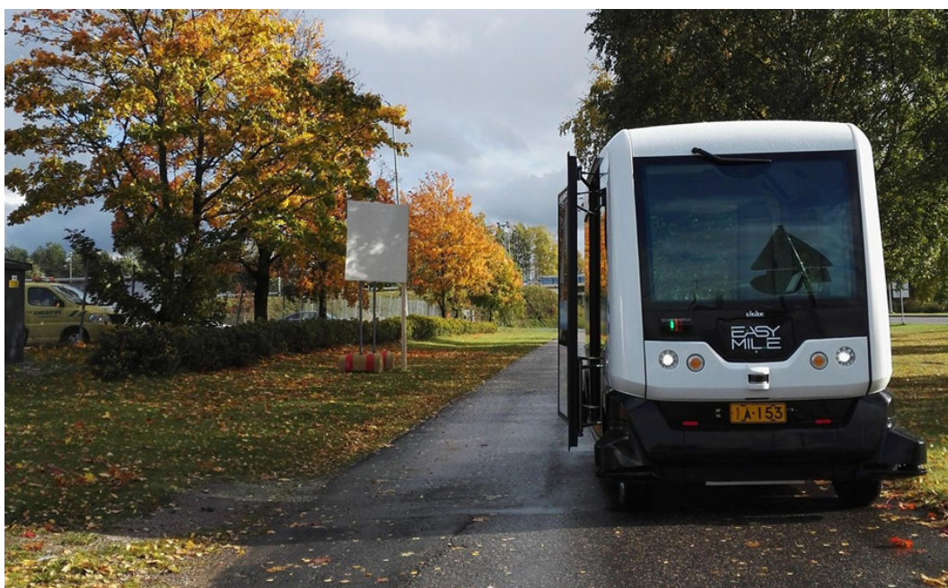
Figure 14. Localization signs were needed in Helsinki route, there wasn't enough fixed structures in the end of the path.
