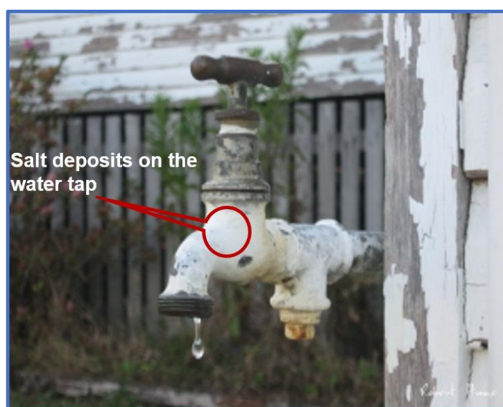
Figure 1. A picture showing public water tap with a salt deposit in the Thulamela Local Municipality, Limpopo Province. The picture was taken on 18 May 2017.
