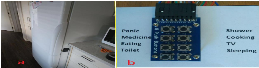
Figure 7. (a) Contact sensing unit connected to fridge door and (b) Manual push button indicator.
