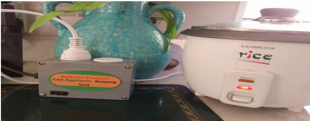
Figure 4. Electronic and electrical (E & E) sensing unit monitoring and controlling rice cooker usage.
