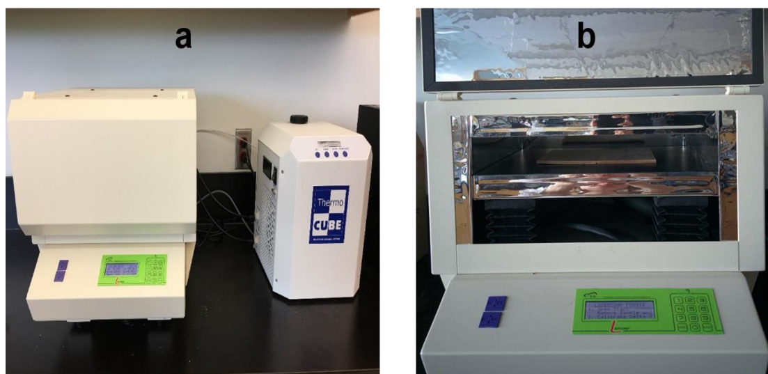
Figure 3. (a) Thermal conductivity testing apparatus; (b) Position of the sample and two heating plates.
