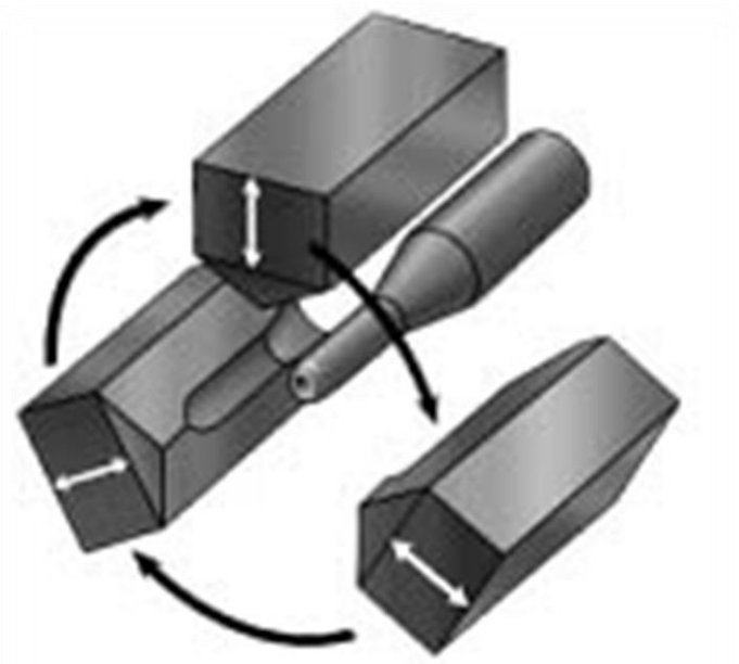
Figure 1. Schematic figure of swaging process.
