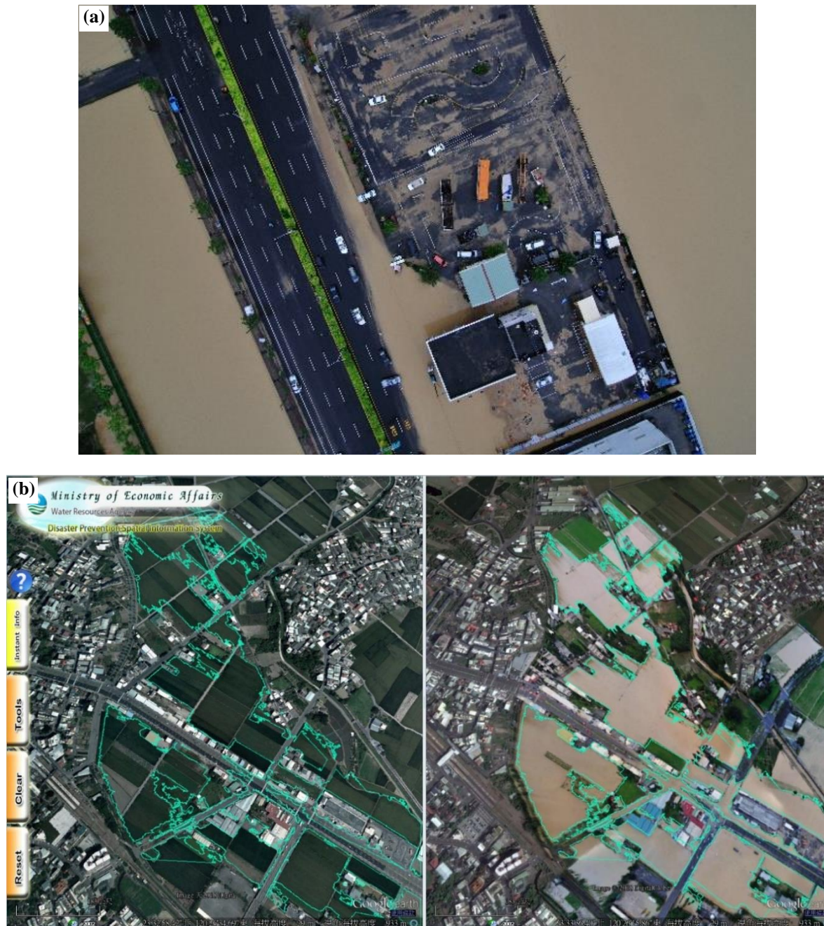
Figure 2. Illustration of the feasibility of mapping the inundated areas with a low-cost UAV. (a) One of the 74 high-spatial-resolution photographs taken by an UAV in Minxiong, Chiayi County in Taiwan on August 29, 2013. The boundary of the inundated area caused by Typhoon Kong-Rey can be clearly delineated from these photographs, and (b) the seamless, color-balanced, and georeferenced mosaic was published on FPERS in dual-window mode (left: before-flood; right: after-flood) within 24 hours.
