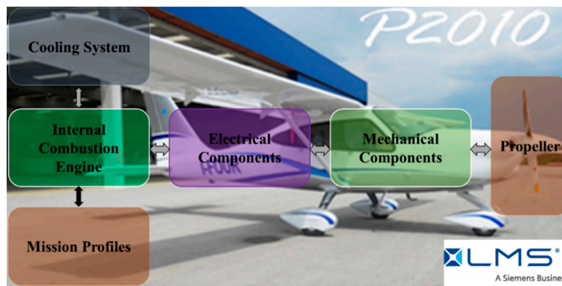
198 Figure 3. Structure of the lumped parameter model of the Hybrid-Electric Propulsion System.
