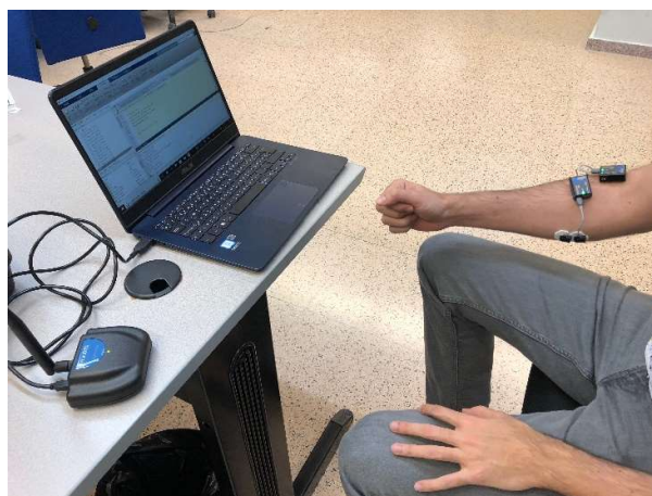
Figure 2. sEMG system acquiring data from a subject.
