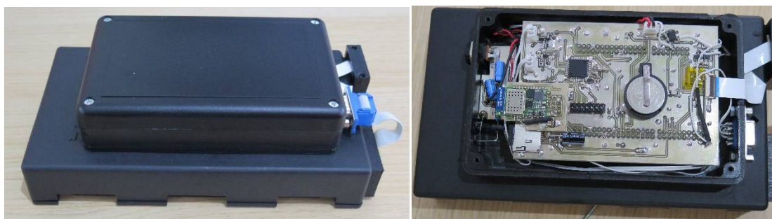
Fig. 1. (Left) A prototype of the smart trap. (Right) The electronics are mounted on top of a plastic trap.
