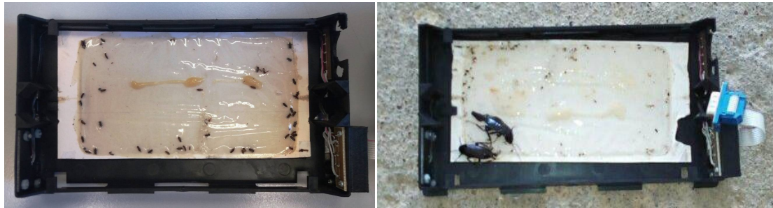
Fig. 4. Evaluation of reported results. Sticky surface inside the trap after 2 days of placement in (left) a cereal grain storage facility with serious insect infestations, (right) in an old food warehouse with an increased presence of cockroaches.
