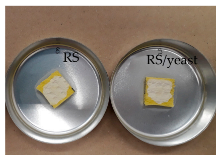
Figure S2. Water soaked sponges with different types of coatings. On the left it is evident the drying region around the sponge due to the water loss.
