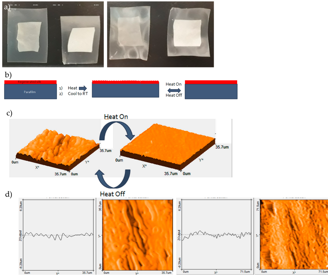
Figure 6. (a) Photographs of RS/yeast/paraffin and RS/paraffin bilayer systems before (left) and after (right) the wrinkle activation. (b) Schematic illustration of temperature driven wrinkling. The bilayer system is flat at room temperature, the heat induces the temperature increasing and thus the thermal expansion of the paraffin substrate, resulting in the increase in the compressive strain of the bilayer systems once cooled down to room temperature with the appearance of the wrinkles. Once the wrinkled state was activated, the heat/temperature can again induce the thermal expansion of the paraffin substrate, resulting in the reversibility of the temperature-driven wrinkles. (c) AFM images showing the reversibility of the temperature-driven wrinkles. (d) AFM images and related profile images of RS (left) and RS/yeast (right) film layers.
