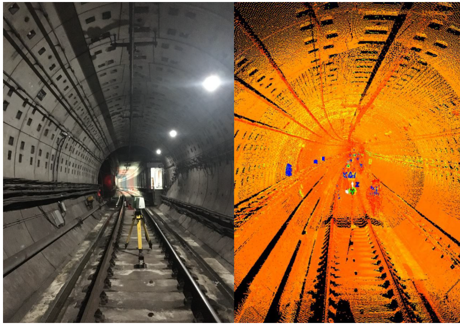
Figure 13. The realistic picture and point cloud of Shanghai metro line 7 scanned by TLS in this monitoring project. There is a Leica C10 scanstation in tunnel
