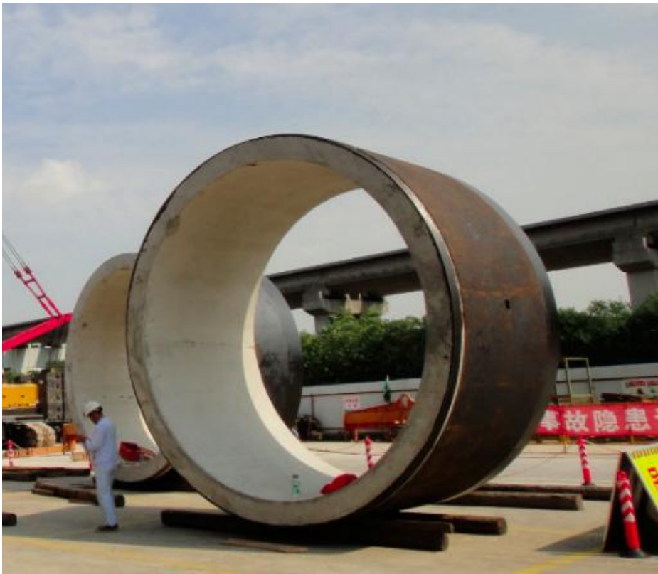
Figure 10. The pipe-jacking tunnel lining used in the experiment
