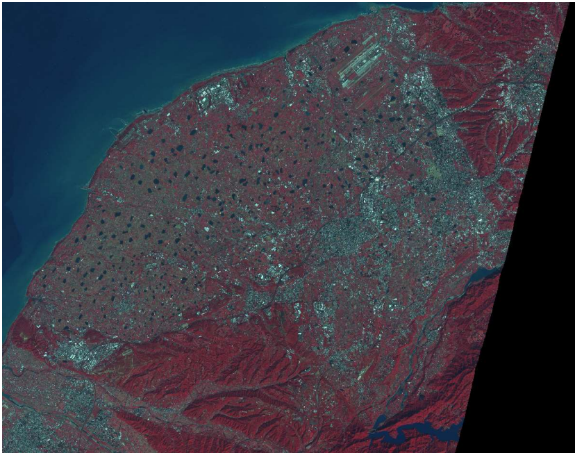
Figure 4. SPOT 5 Pseudo-color image of the study area acquired in November, 2014. The green, red, and near infrared bands are displayed in blue, green, and red colors, respectively, in the pseudo-color image.
