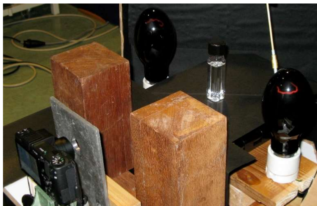
Figure 14. The set-up used to monitor, in situ , the fluorescence of an RFG gel on insertion of a seed of ^{192}\text{Ir} . The main constituents are a 20 \times 20 \text{ mm}^2 glass cell containing the gel into which a 1.9 mm diameter catheter (shown in Figure 15) is inserted via a septum cap ; two mercury-arc UV (365 nm) lamps, a Ricoh GX200 digital camera with a lead shield against gamma irradiation and wooden shields against direct UV.
