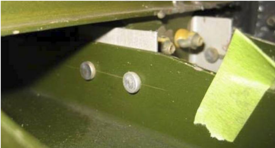
Figure 15. Typical SCC in a P3C (Orion) wing, photograph courtesy of M. Dorman, RAAF MPSO.
