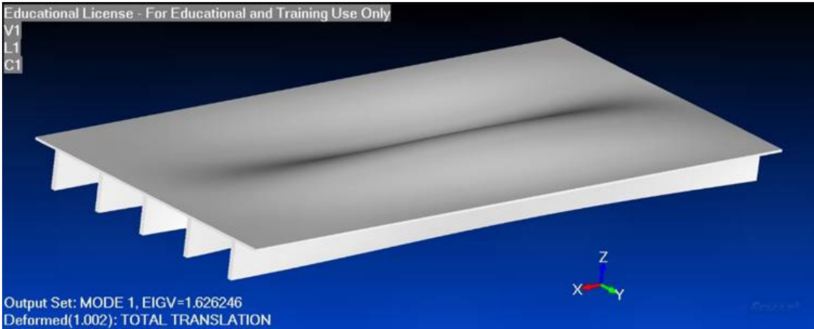
Figure 24 - Buckling loads for the baseline panels (no corrosion), from [44].
