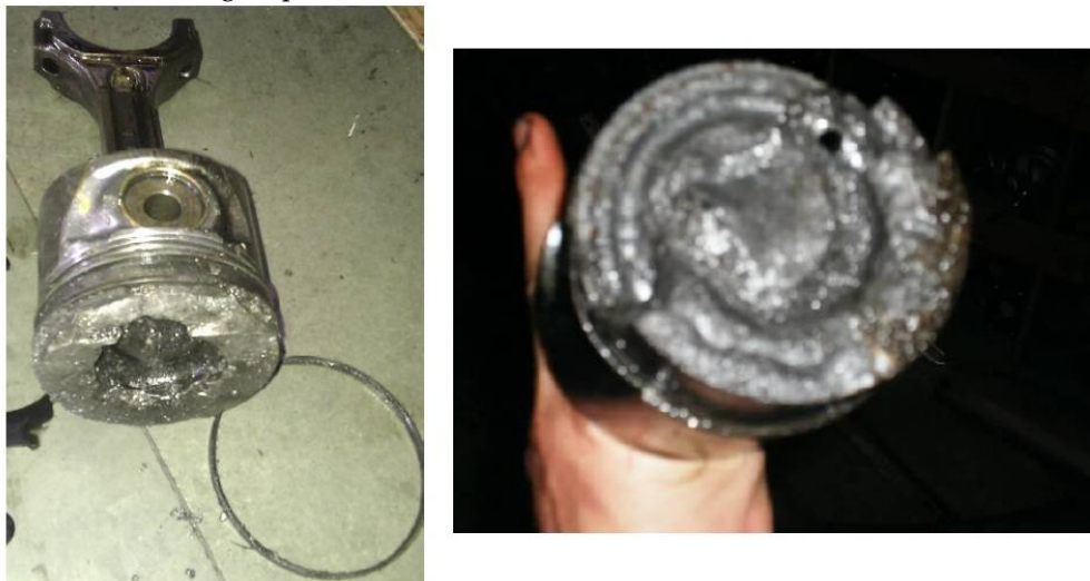
Figure 3: Severe overheating failure of engine piston [9].
