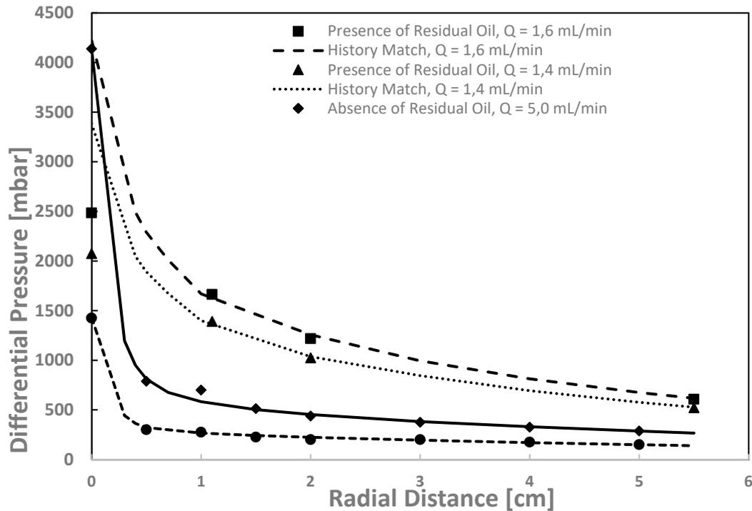
**Figure 8:** Differential pressure profiles for 2000-ppm 3630S HPAM floods in presence and absence of residual oil in radial geometry as a function of distance from injector to producer for four flow rates.
