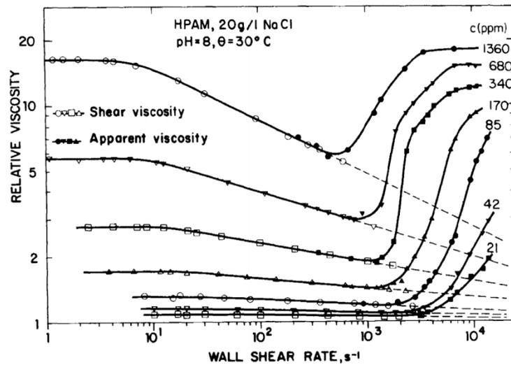
**Figure 2:** Effect of polymer concentration on the onset of extensional viscosity in a model with 45 successive constrictions<sup>[33]</sup>
