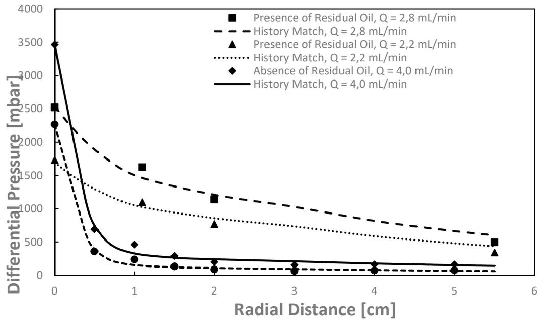
**Figure 6:** Differential pressure profiles for 800-ppm HPAM floods in presence and absence of residual oil in radial geometry as a function of distance from injector to producer for four flow rates.
