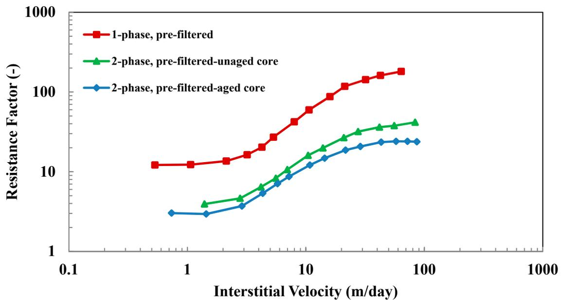
**Figure 5:** Resistance factor versus interstitial velocity of 500 ppm pre-filtered FP3630S HPAM polymer dissolved in 1 wt% NaCl brine, comparison of single phase polymer flow and polymer flow at residual oil saturation.
