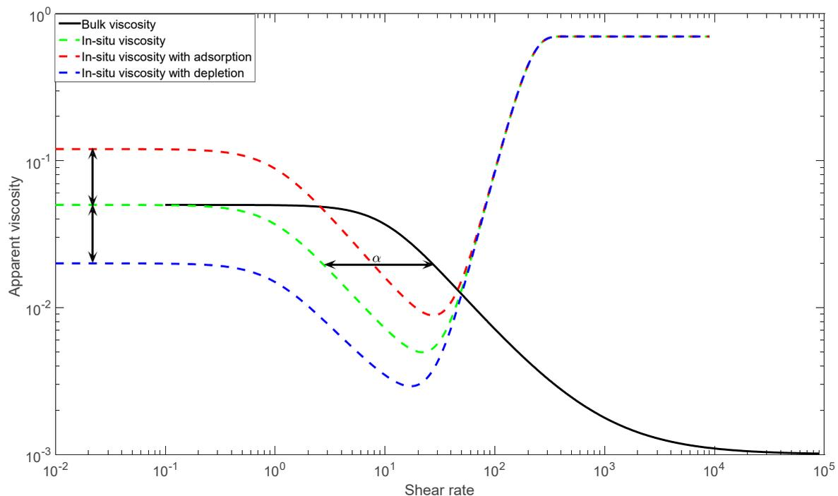
**Figure 1:** schematic comparison of in-situ and bulk rheology
