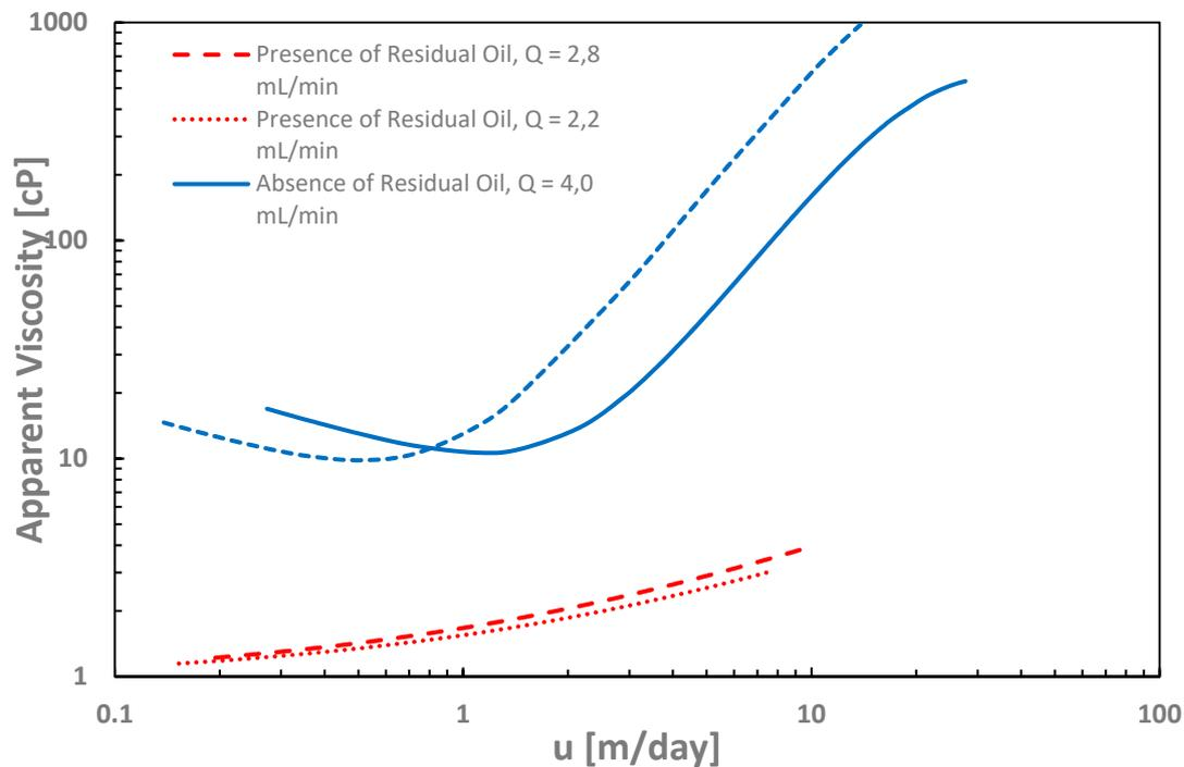
**Figure 7:** Apparent viscosity from history match of differential pressure for 800-ppm HPAM in presence and absence of residual oil in radial geometry.
