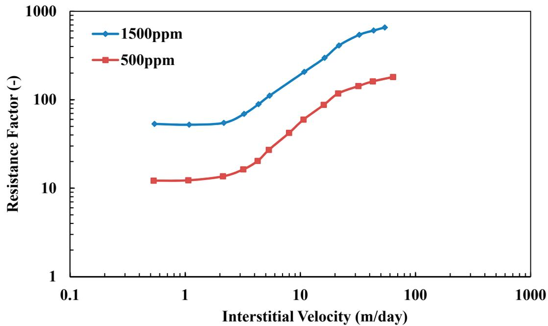
**Figure 4** Resistance factor versus interstitial velocity of pre-filtered FP3630S HPAM polymer dissolved in 1 wt% NaCl brine.
