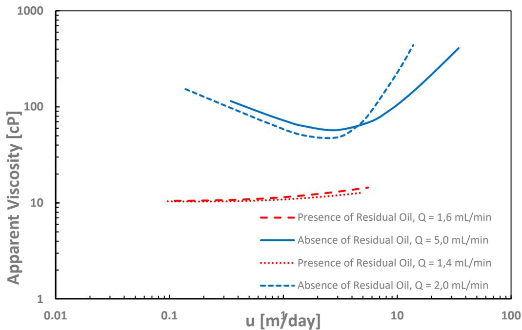
**Figure 9:** Apparent viscosity from history match of differential pressure for 2000-ppm 3630S HPAM in presence and absence of residual oil in radial geometry.
