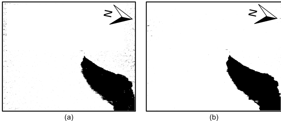
Figure 5. ASM-based oil detection maps relevant to the CSK SAR scene collected on 23 April 2010. (a) HH and (b) VV channel.
