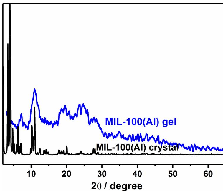
**Fig. S3.** Powder XRD patterns of the as-synthesized MIL-100(Al) gels and the XRD pattern simulated from crystal structure data of MIL-100(Al). The result of the as-synthesized MIL-100(Al) gels agrees well with the simulated result of single-crystal MIL-100(Al).
