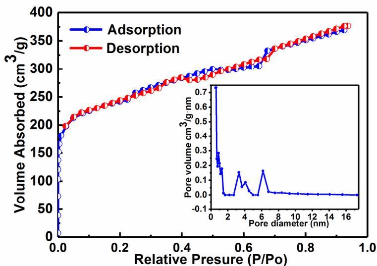
**Fig. S4.** Nitrogen adsorption-desorption isotherm of MIL-100(Al) gel measured at 77 K. The inset shows the corresponding pore size distribution analysis obtained using Discrete Fourier Transform (DFT) method. The BET surface area and pore volume of the MOGs were calculated to be 920 m<sup>2</sup>/g and 0.535 cm<sup>3</sup>/g, respectively. The large surface area and high porosity make this material to be possibly used for highly efficient drug loading.
