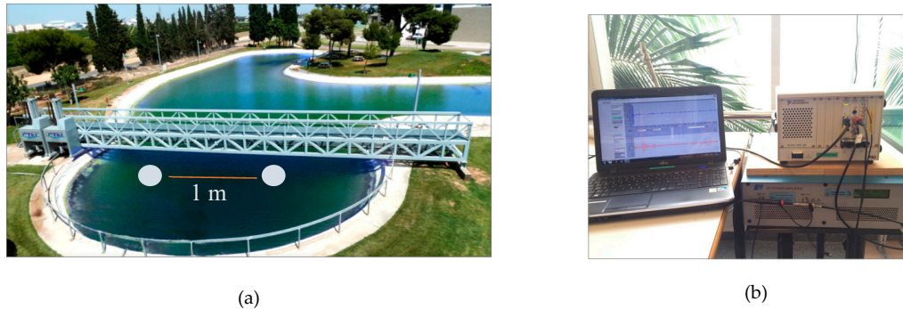
Figure 1. Pictures of the experimental setup. (a) The lake where the position of transducers is indicated by white circles. (b) Equipment used for the calibrations and measurements.
