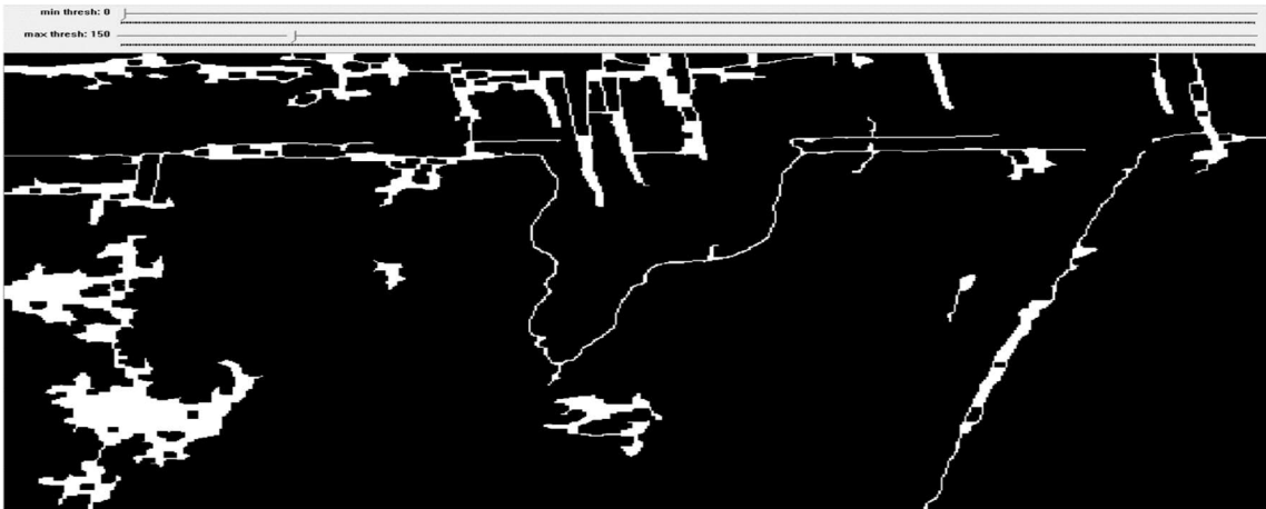
Figure 20. Resulting image obtained from top-hat morphological operation
