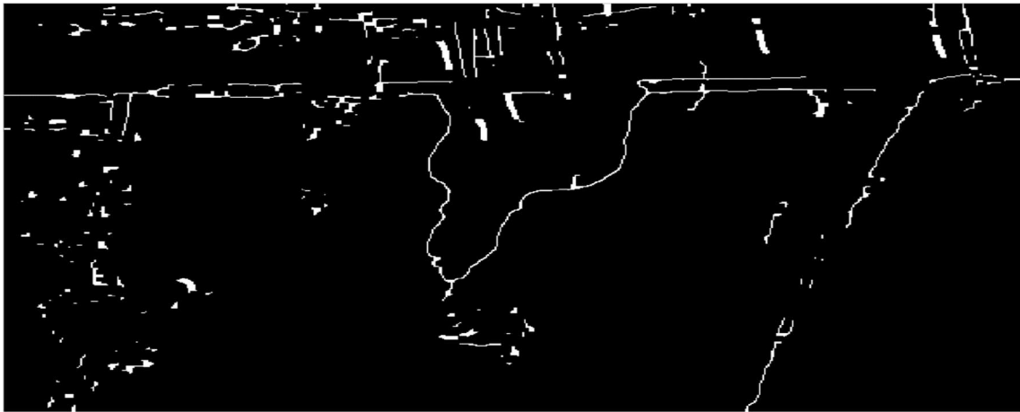
Figure 19. Resulting image obtained from Canny edge detection
