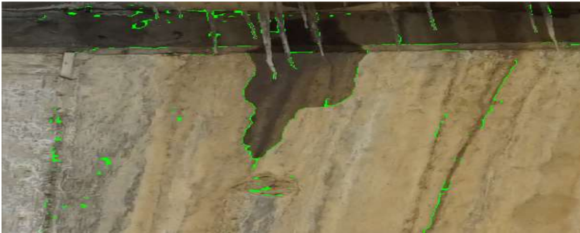
Figure 21. Resulting image obtained from water leak detection
