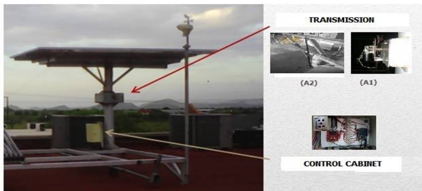
Figure 11. Solar tracker prototype and components.
