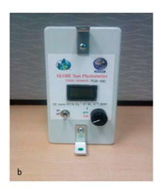
**Figure2.**The GLOBE hand held sun photometer. (a) Basic circuit of the GLOBE sun photometer, (b) A fully assembled sun photometer.
