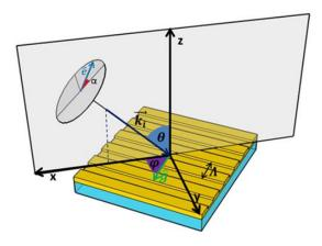
Figure 1. Conical mounting scheme
