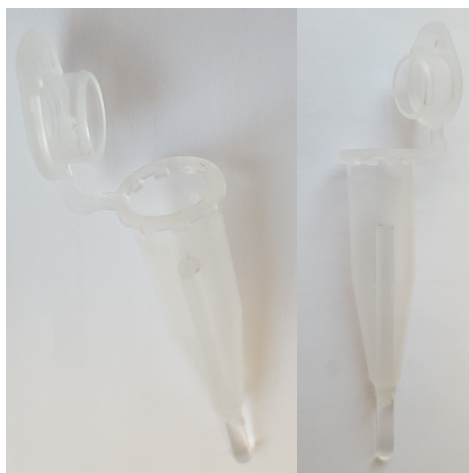
Figure 7. Image of eppendorf tube with glass rod inside used for photopolymerizing pre-gel in squalane-PI.
