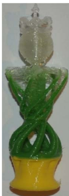
215 Figure 5. Model produced after two filament advance problems
