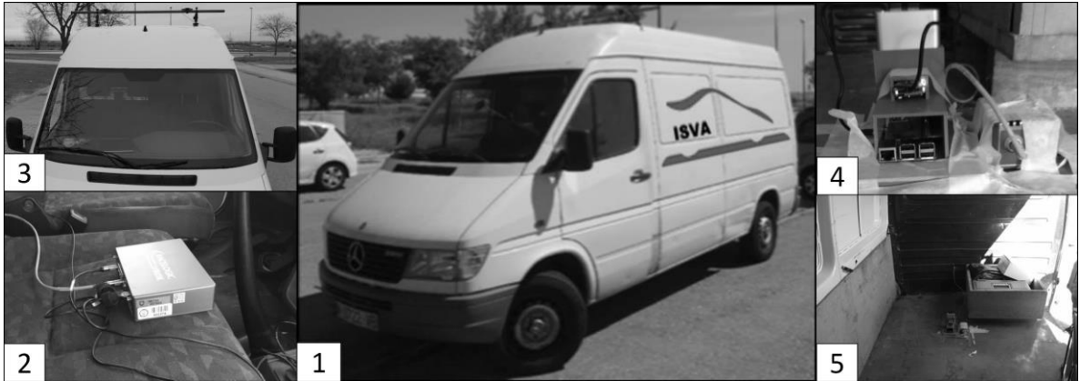
Figure 1. Test vehicle (1) equipped with different low-cost systems (4, 5), VBOX data logger, 3 IMU sensors (2) and GPS dual-antenna (3).
