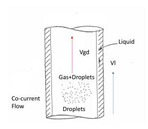
Figure 2. Two Phase Upward Co-current Annular Flow
