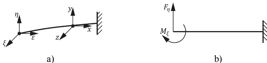
Figure 3. a) Local coordinates of the beam for potential energy evaluation; b) local generalized coordinates of the beam.
