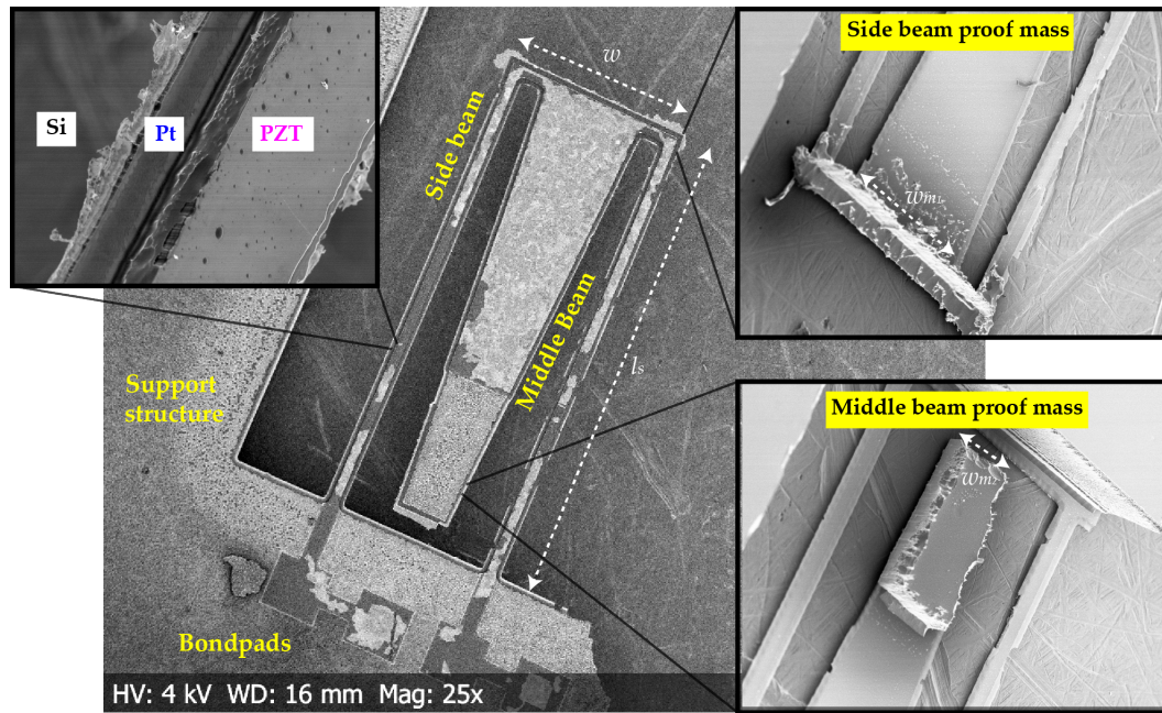
Figure 9. SEM image of M-shape at 25\times magnification. Insets contain the backside processed images of the primary and secondary proof masses, and the PZT layer on the bottom electrodes on the side-beam cantilevers
