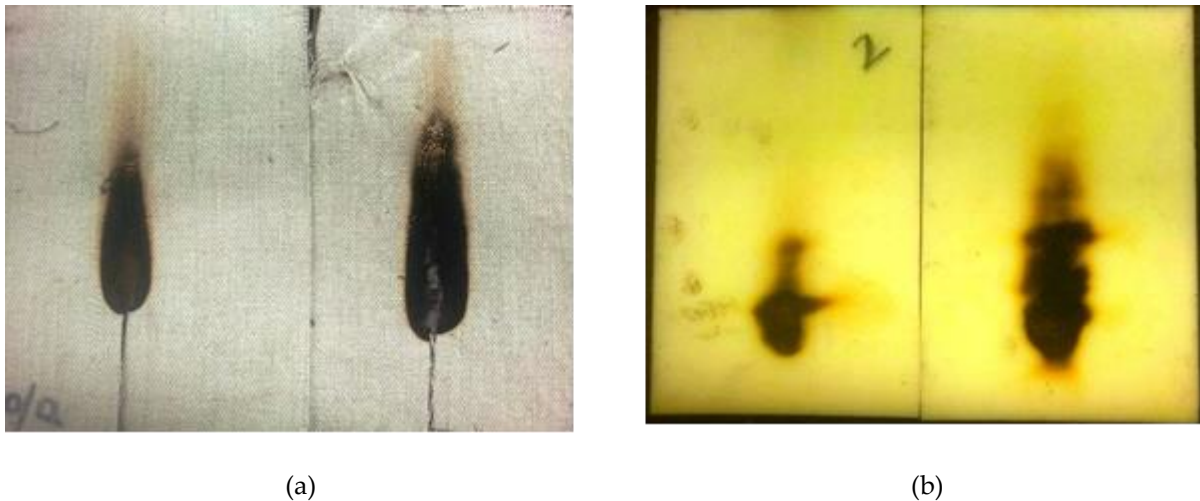
264 Figure 3: Composite fabric/foam specimens after small-scale simulated match testing (a) sample 6 265 fabric; (b) PU foam underlying sample 2, before (left) and after (right) water-soaking.
