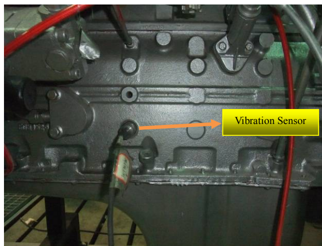
Figure 6. Measuring position of vibration sensor.
