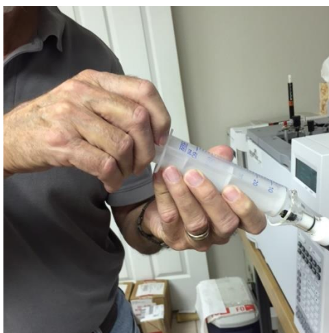
Figure 18. Whole air fraction collection process of high-impact odorants from the sniff port for off-line odor assessment.
