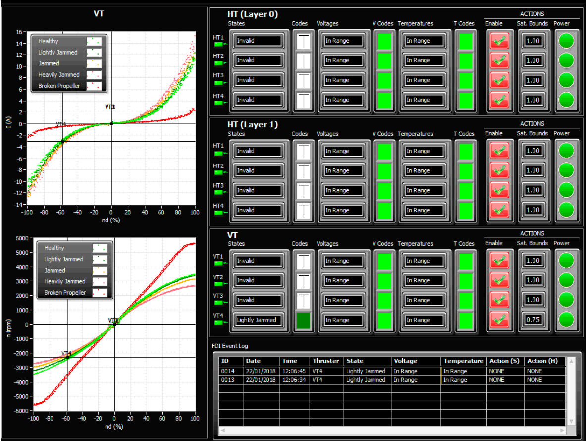
Figure 17. Thruster FDI result for thruster state = "Lightly Jammed".
