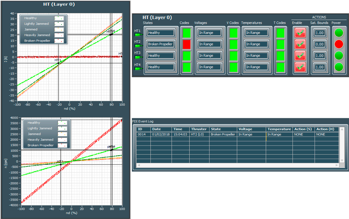
Figure 24. Test 2 (Closed-Loop): Total fault in HT2 (“Broken Propeller”) with disabled fault accommodation.
