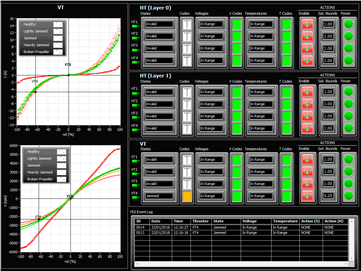
Figure 18. Thruster FDI result for thruster state = "Jammed".
