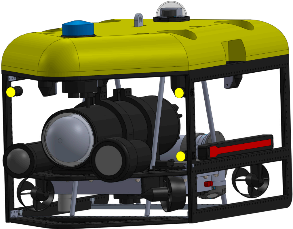
Figure 1. Observation class IROV, developed by CRIS researchers, UL.
