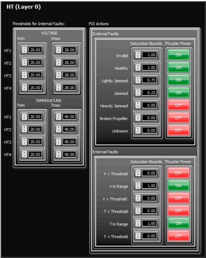
Figure 13. Fault Code Table for horizontal thrusters (Layer 0).
