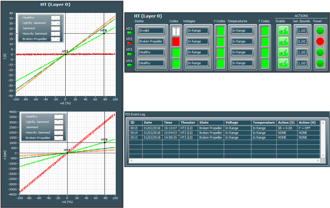
Figure 26. Test 3 (Closed-Loop): Total fault in HT2 (“Broken Propeller”) with enabled fault accommodation.
