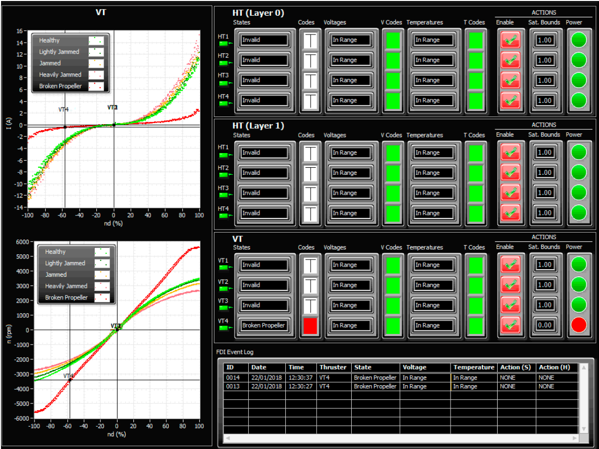
Figure 20. Thruster FDI result for thruster state = “Broken Propeller”.
