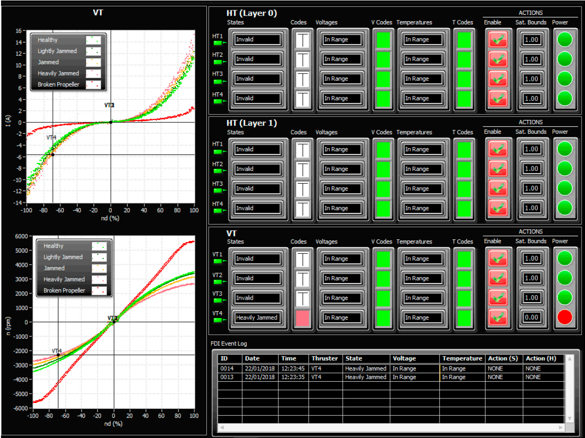
Figure 19. Thruster FDI result for thruster state = "Heavily Jammed".
