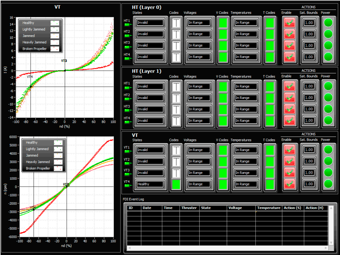
Figure 16. Thruster FDI result for thruster state = "Healthy".
