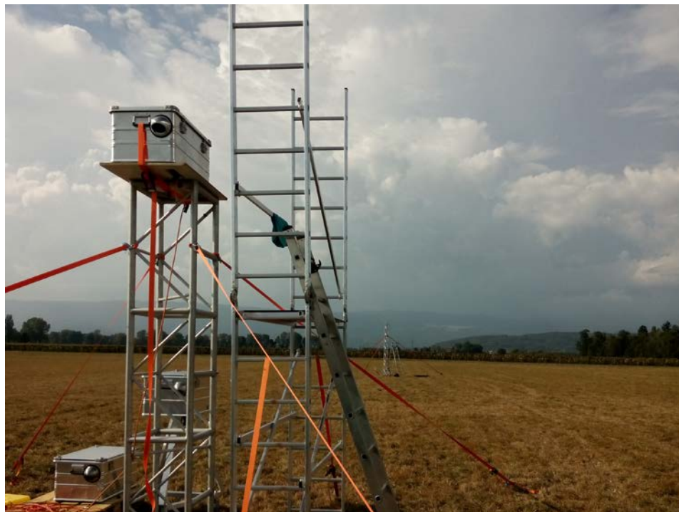
Figure 3. Three miniDOAS instruments located at the release site, 15 m downwind of the source center (position near ). The distances between the boxes containing the light source and the detector (picture foreground) and the reflectors (picture background) were approx. 35 m. The measurement heights were 0.5 m ( near/bottom ), 1.25 m ( near/middle ) and 3.0 m ( near/top ) above ground.
