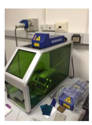
72 Figure 6: 1070 nm Yb-doped pulsed fiber laser (AREX 20, Datalogic, Italy).
