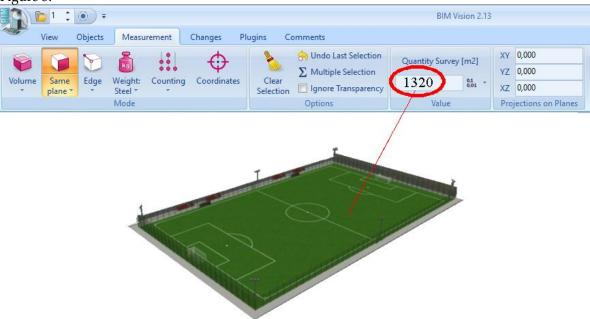
**Figure 3.** Take-off procedure in the ICE-MACRO method based on the MACRO BIM model - view in the BIM Vision browser
