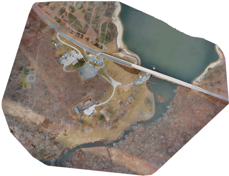
Figure 3. Orthomosaic generated using the fixed wing imagery dataset.
