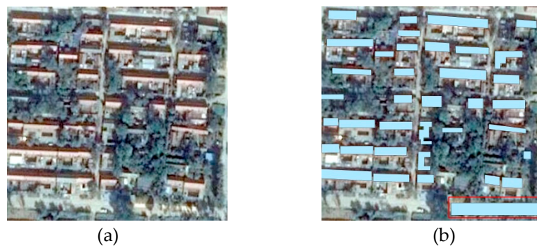
Figure 9. Another testing image: (a) The original image. (b) Labeled result. A section of road marked in the red rectangle is wrongly labeled as a building
