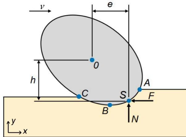
**Fig. S1.** Schematic of forces on an ellipsoidal abrasive particle in three-body abrasion.
